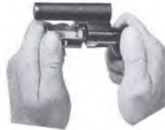
Fig. 33 Removing the bolt assembly components
